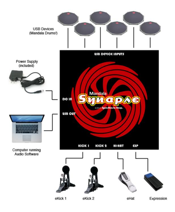
Fig. 1) Typical Synapse Setup
